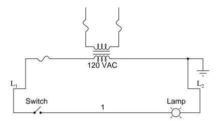
Here, the lamp (load) is located on the right-hand side of the rung, and so is the ground connection for the power source. This is no accident or coincidence; rather, it is a purposeful element of good design practice. Suppose that wire #1 were to accidently come in contact with ground, the insulation of that wire having been rubbed off so that the bare conductor came in contact with grounded, metal conduit. Our circuit would now function like this:
