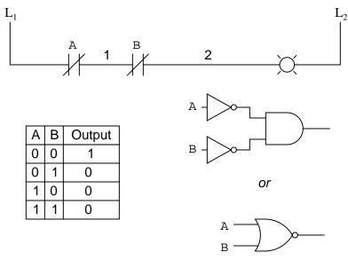
A pattern quickly reveals itself when ladder circuits are compared with their logic gate counterparts:
