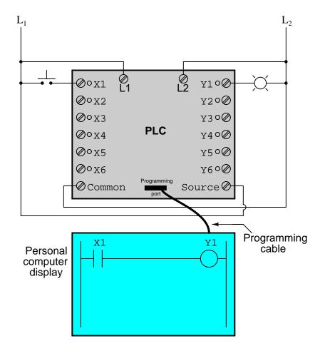
When the pushbutton switch is unactuated (unpressed), no power is sent to the X1 input of the PLC. Following the program, which shows a normally-open X1 contact in series with a Y1 coil, no "power" will be sent to the Y1 coil. Thus, the PLC's Y1 output remains de-energized, and the indicator lamp connected to it remains dark.
