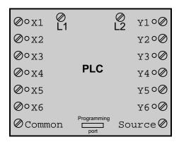
Inside the PLC housing, connected between each input terminal and the Common terminal, is an opto-isolator device (Light-Emitting Diode) that provides an electrically isolated "high" logic signal to the computer's circuitry (a photo-transistor interprets the LED's light) when there is 120 VAC power applied between the respective input terminal and the Common terminal. An indicating LED on the front panel of the PLC gives visual indication of an "energized" input:
