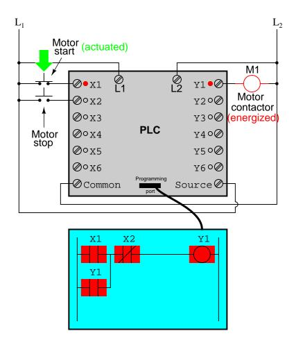
Now, if we release the "Start" pushbutton, the normally-open X1 "contact" will return to its "open" state, but the motor will continue to run because the Y1 seal-in "contact" continues to provide "continuity" to "power" coil Y1, thus keeping the Y1 output energized:
