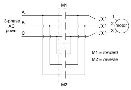
When contactor  $M_1$  is energized, the 3 phases (A, B, and C) are connected directly to terminals 1, 2, and 3 of the motor, respectively. However, when contactor  $M_2$  is energized, phases A and B are reversed, A going to motor terminal 2 and B going to motor terminal 1. This reversal of phase wires results in the motor spinning the opposite direction. Let's examine the control circuit for these two contactors:
