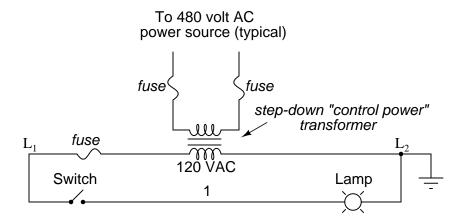
Typically in industrial relay logic circuits, but not always, the operating voltage for the switch contacts and relay coils will be 120 volts AC. Lower voltage AC and even DC systems are sometimes built and documented according to "ladder" diagrams:
