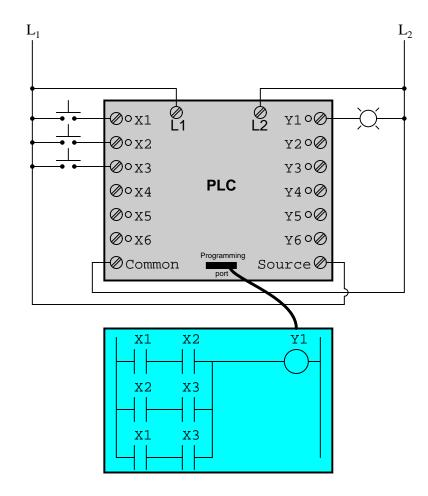
To build an equivalent circuit using electromechanical relays, three relays with two normallyopen contacts each would have to be used, to provide two contacts per input switch. Using a PLC, however, we can program as many contacts as we wish for each "X" input without adding additional hardware, since each input and each output is nothing more than a single bit in the PLC's digital memory (either 0 or 1), and can be recalled as many times as necessary.
