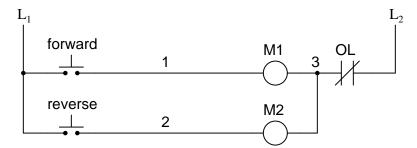
Take note of the normally-closed "OL" contact, which is the thermal overload contact activated by the "heater" elements wired in series with each phase of the AC motor. If the heaters get too hot, the contact will change from its normal (closed) state to being open, which will prevent either contactor from energizing.
