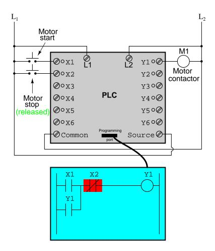
An important point to make here is that *fail-safe* design is just as important in PLC-controlled systems as it is in electromechanical relay-controlled systems. One should always consider the effects of failed (open) wiring on the device or devices being controlled. In this motor control circuit example, we have a problem: if the input wiring for X2 (the "Stop" switch) were to fail open, there would be no way to stop the motor!
