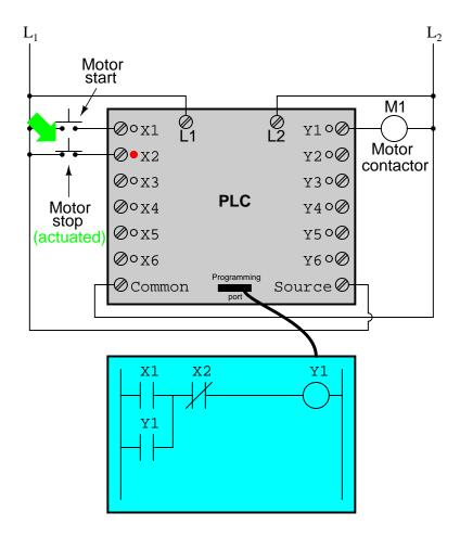
When the "Stop" pushbutton is released, input X2 will de-energize, returning "contact" X2 to its normal, "closed" state. The motor, however, will not start again until the "Start" pushbutton is actuated, because the "seal-in" of Y1 has been lost:
