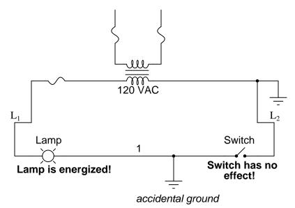
This time the accidental grounding of wire #1 will force power to the lamp while the switch will have no effect. It is much safer to have a system that blows a fuse in the event of a ground fault than to have a system that uncontrollably energizes lamps, relays, or solenoids
