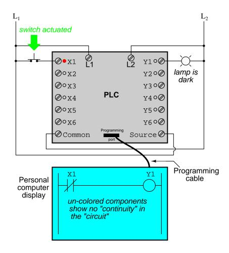
One of the advantages of implementing logical control in software rather than in hardware is that input signals can be re-used as many times in the program as is necessary. For example, take the following circuit and program, designed to energize the lamp if at least two of the three pushbutton switches are simultaneously actuated:
