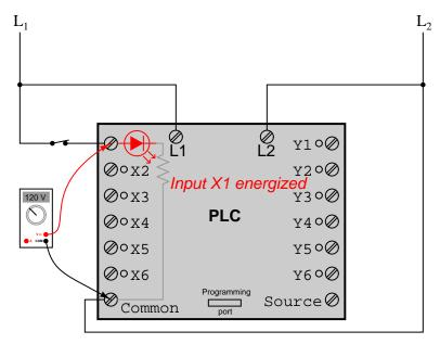
Output signals are generated by the PLC's computer circuitry activating a switching device (transistor, TRIAC, or even an electromechanical relay), connecting the "Source" terminal to
