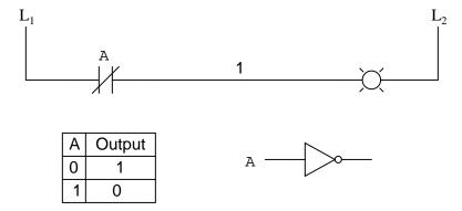
Now, the lamp energizes if the contact is *not* actuated, and de-energizes when the contact *is* actuated.
