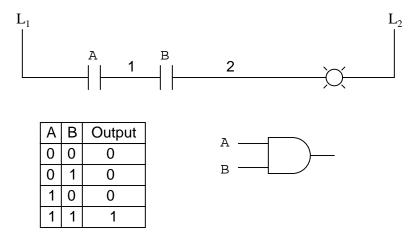
Now, the lamp energizes only if contact A *and* contact B are simultaneously actuated. A path exists for current from wire  $L_1$  to the lamp (wire 2) if and only if *both* switch contacts are closed.
