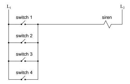
Essentially, this is the OR logic function implemented with four switch inputs. We could expand this circuit to include any number of switch inputs, each new switch being added to the parallel network, but I'll limit it to four in this example to keep things simple. At any rate, it is an elementary system and there seems to be little possibility of trouble.
