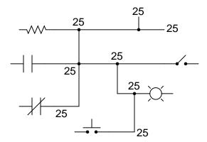
In ladder diagrams, the load device (lamp, relay coil, solenoid coil, etc.) is almost always drawn at the right-hand side of the rung. While it doesn't matter electrically where the relay coil is located within the rung, it *does* matter which end of the ladder's power supply is grounded, for reliable operation.
