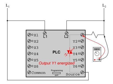
In this way, the PLC is able to interface with real-world devices such as switches and solenoids.
