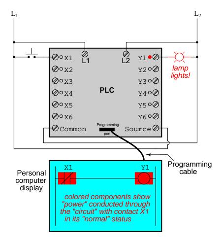
In this next illustration, the switch is shown actuated (pressed):
