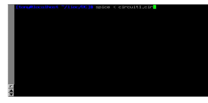
As soon as you press the [Enter] key to issue this command, text from SPICE's output should scroll by on the computer screen. Here is a screenshot showing what SPICE outputs on my computer (I've lengthened the "terminal" window to show you the full text. With a normal-size terminal, the text easily exceeds one page length):
