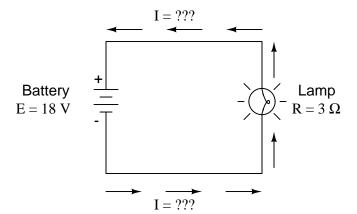
In the above circuit, we know we have a battery voltage of 18 volts and a lamp resistance of 3  $\Omega$ . Using Ohm's Law to determine current, we get:
