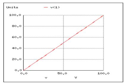
Note how Nutmeg plots the resistor voltage v(1) (voltage between node 1 and the implied reference point of node 0) as a line with a positive slope (from lower-left to upper-right).
