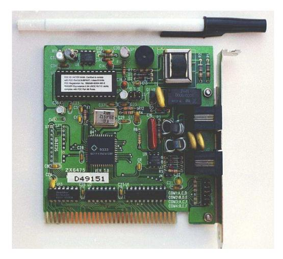
This particular circuit board is a computer accessory called a "modem," which allows digital information transfer over telephone lines. There are at least a dozen resistors (all rated at 1/4 watt power dissipation) that can be seen on this modem's board. Every one of the black rectangles (called "integrated circuits" or "chips") contain their own array of resistors for their internal functions, as well.
