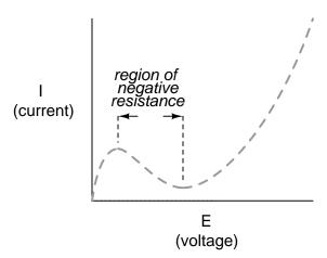
Most notably, high-vacuum electron tubes known as *tetrodes* and semiconductor diodes known as *Esaki* or *tunnel* diodes exhibit negative resistance for certain ranges of applied voltage.
