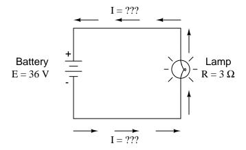
Now, the battery voltage is 36 volts instead of 18 volts. The lamp is still providing 3  $\Omega$  of electrical resistance to the flow of electrons. The current is now:
