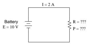
All we've been given here to start with is the battery voltage (10 volts) and the circuit current (2 amps). We don't know the resistor's resistance in ohms or the power dissipated by it in watts. Surveying our array of Ohm's Law equations, we find two equations that give us answers from known quantities of voltage and current:
