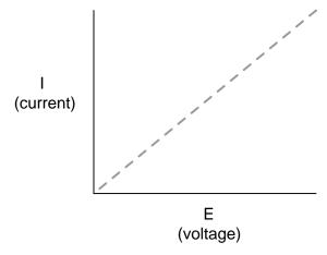
The straight-line plot of current over voltage indicates that resistance is a stable, unchanging value for a wide range of circuit voltages and currents. In an "ideal" situation, this is the case. Resistors, which are manufactured to provide a definite, stable value of resistance, behave very much like the plot of values seen above. A mathematician would call their behavior "linear."
