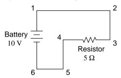
Here, we only have 2 components excluding the wires: the battery and the resistor. Though the connecting wires take a convoluted path in forming a complete circuit, there are several electrically common points in the electrons' path. Points 1, 2, and 3 are all common to each other, because they're directly connected together by wire. The same goes for points 4, 5, and 6.
