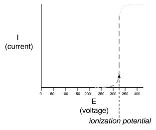
The graph shown is approximate for a small air gap (less than one inch). A larger air gap would yield a higher ionization potential, but the shape of the I/E curve would be very similar: practically no current until the ionization potential was reached, then substantial conduction after that.
