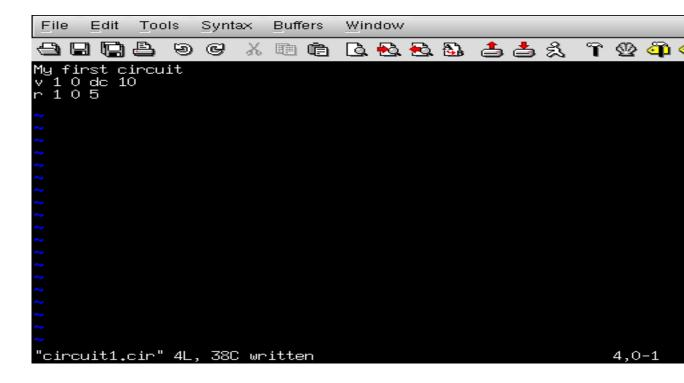
Now, SPICE will know there is a resistor connected between nodes 1 and 0 with a value of 5  $\Omega$ . This very brief line of text tells the computer we have a resistor ("r") connected between the same two nodes as the battery (1 and 0), with a resistance value of 5  $\Omega$ .
