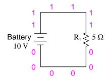
In the above illustration, I've shown multiple "1" and "0" labels around each respective wire to emphasize the concept of common points sharing common node numbers, but still this is a graphic image, not a text description. SPICE needs to have the component values and node numbers given to it in text form before any analysis may proceed.
