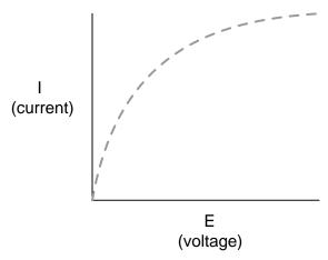
The plot is no longer a straight line. It rises sharply on the left, as voltage increases from zero to a low level. As it progresses to the right we see the line flattening out, the circuit requiring greater and greater increases in voltage to achieve equal increases in current.
