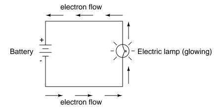
In the above circuit, there is only one source of voltage (the battery, on the left) and only one source of resistance to current (the lamp, on the right). This makes it very easy to apply Ohm's Law. If we know the values of any two of the three quantities (voltage, current, and resistance) in this circuit, we can use Ohm's Law to determine the third.
