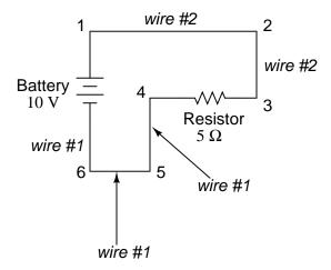
Points 1, 2, and 3 are all common to each other, so the wire connecting point 1 to 2 is labeled the same (wire 2) as the wire connecting point 2 to 3 (wire 2). In a real circuit, the wire stretching from point 1 to 2 may not even be the same color or size as the wire connecting point 2 to 3, but they should bear the exact same label. The same goes for the wires connecting points 6, 5, and 4.
