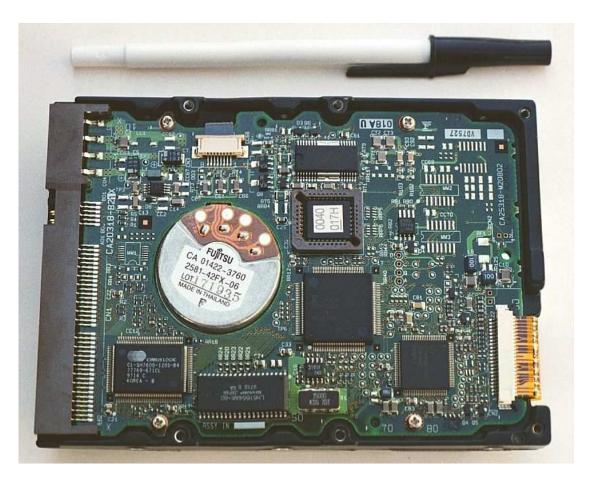
There are over one hundred surface-mount resistors on this circuit board, and this count of course does not include the number of resistors internal to the black "chips." These two photographs should convince anyone that resistors – devices that "merely" oppose the flow of electrons – are very important components in the realm of electronics!
