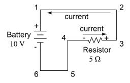
We could make our table of voltages a little more complete by marking the polarity of the voltage for each pair of points in this circuit:
